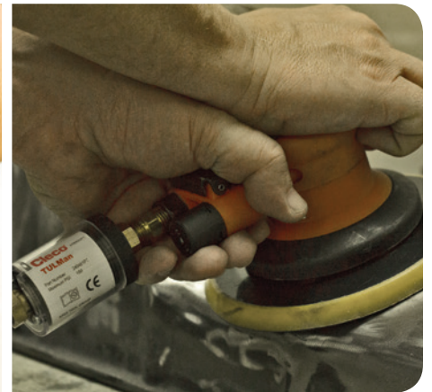
Run time monitoring for consumable use or process efficiency
