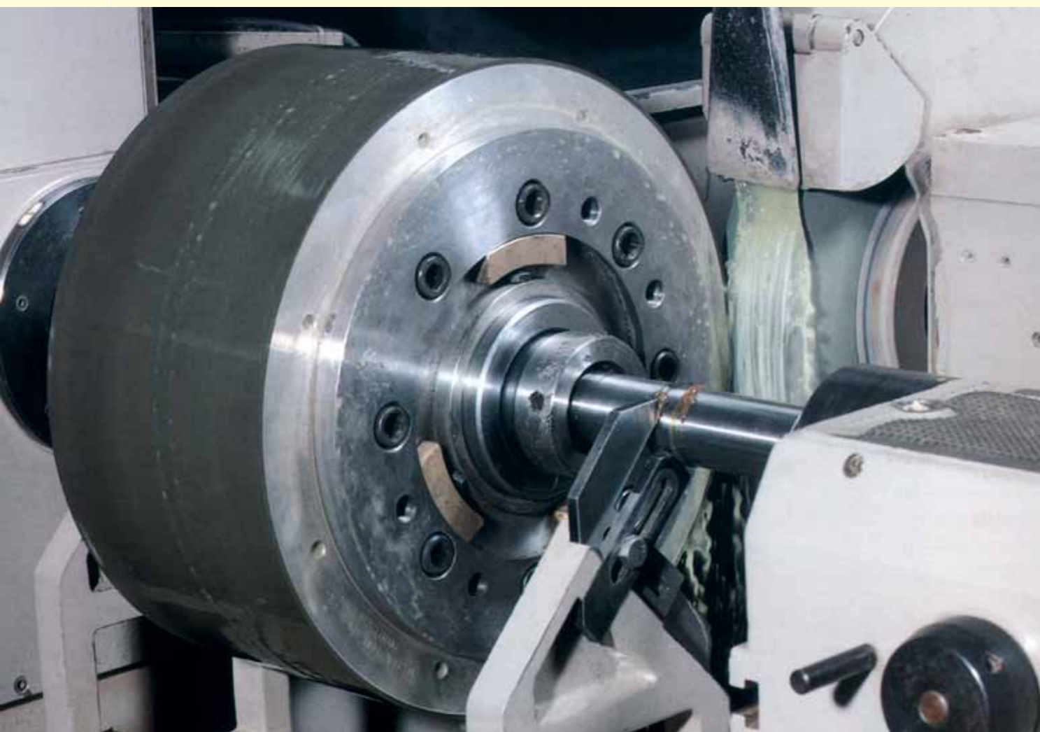
Truing of resin bonded centerless wheel
