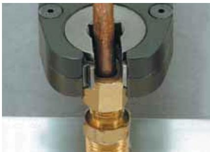
*Make sure that the socket is set to the open position. If not, push the throttle lever down half way to release the socket back to the open position.*
