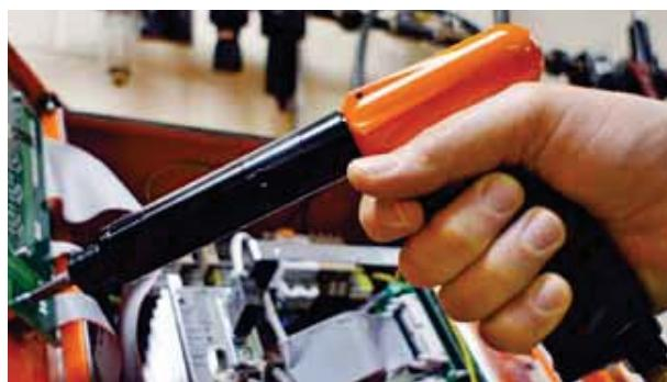
The "P" handle is best suited for thread cutting fasteners where force must be exerted against the ergonomically shaped "P" handle during the process.
